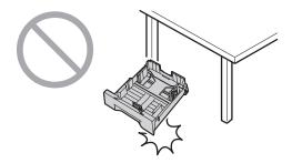
Hold the paper input tray with both hands when removing or installing. The paper input tray weighs approximately 2 kg when the recording paper is fully installed.
